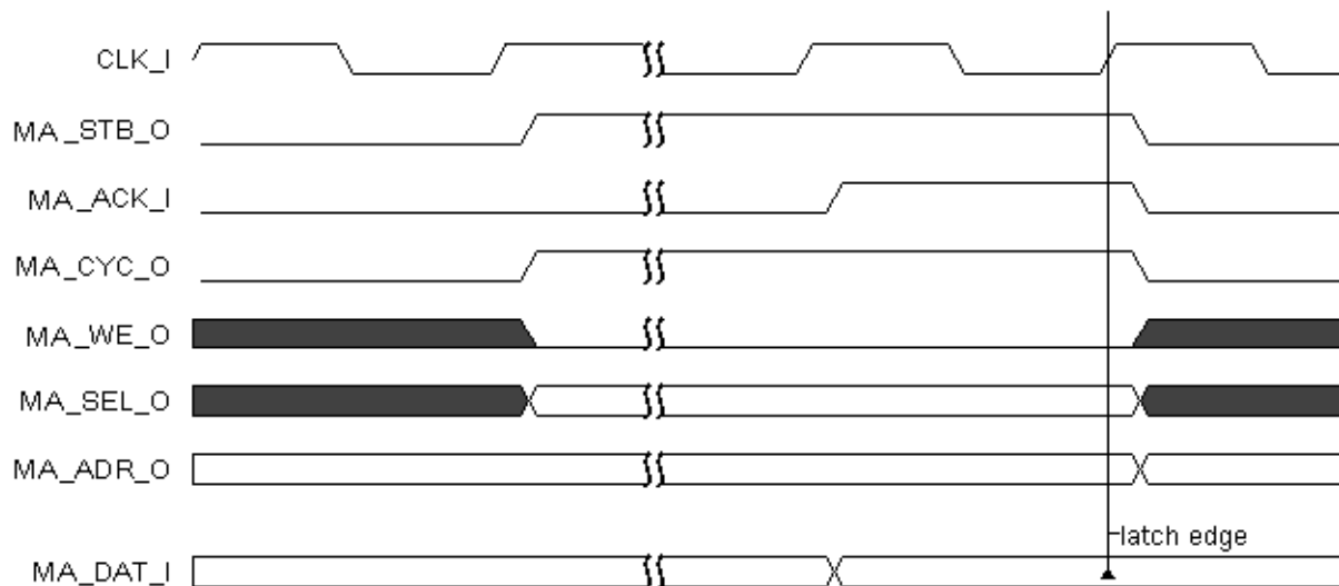
Figure 6: DMA Controller Reading Data from Source Address
