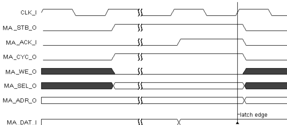
Figure 7: DMA Controller Reading Data from Source Address
